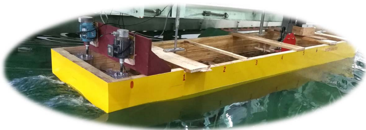
Tank test for straight wing propeller
